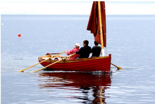
The light clinker version is easy to row
