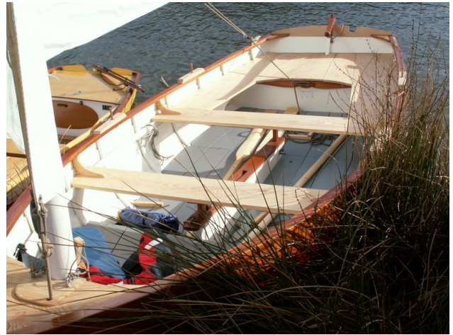
A lot of space, thanks to the lowered centreboard case
