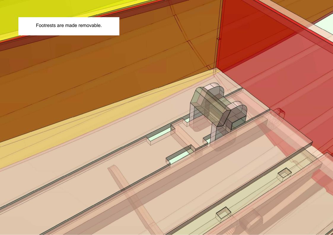
Footrests are built with two plywood cheeks (CNC cut) and two timber parts, each 25 x 50 x 110 mm.
