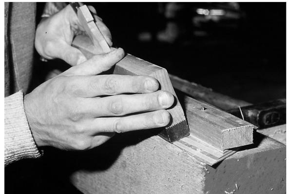
Remember that strakes are usually cut with an extra length of 10 cm about in order to help giving the proper curvature. This extra length is to be taken in account when making end chamfer.
