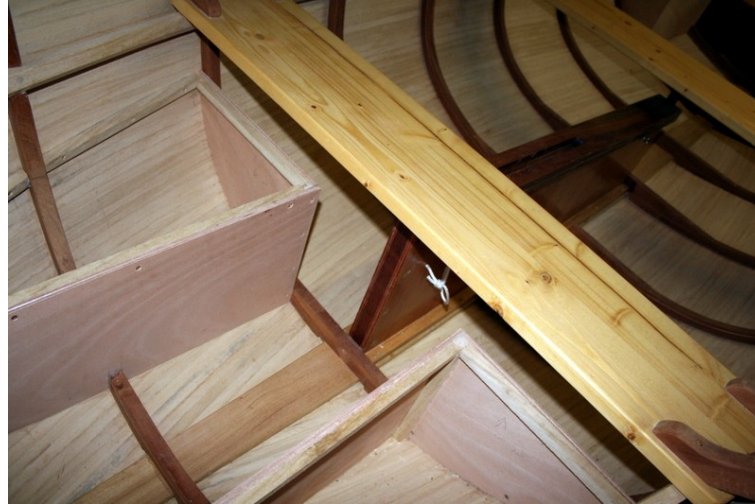
Fore buoyancy tanks showing the centreline space used for oars stowage
