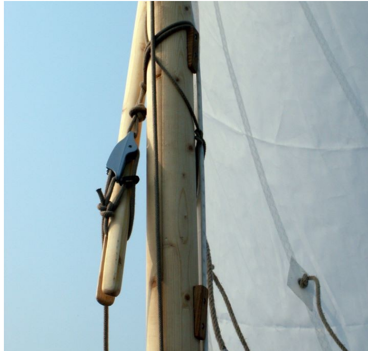
Detail of the snotter arrangement. The clam-cleat allows tuning of the sprit tension
