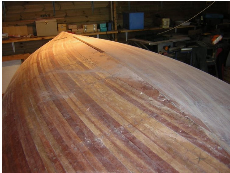
Closing planks, which may be done with several strips glued in advance
