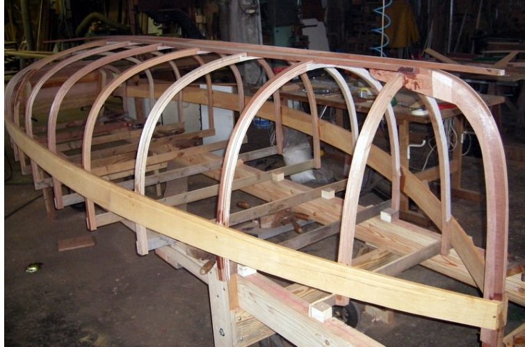
On the picture, the sheerstrake is already fitted and add stiffness to the ensemble
