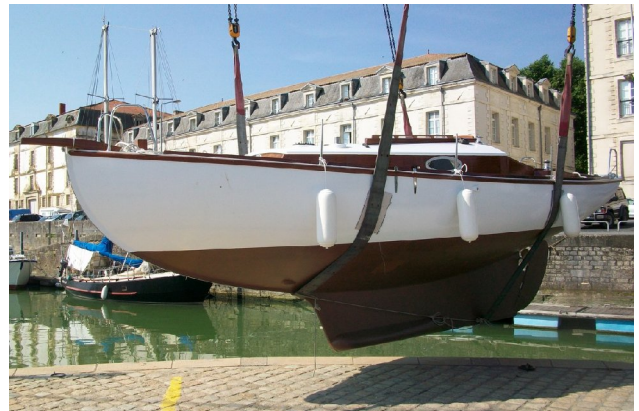
The long keel allows easy drying out. It is thin and fitted with a lead bulb, making the hull very efficient under sail.
