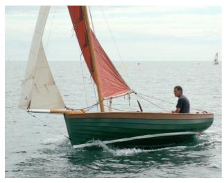
Beg-Meil is a traditional day-boat, gaff sloop rigged, just like many that existed in the old days. It is elegant and seaworthy with its half-deck and varnished wood coamings. A steel pivoting centreboard (40 kg) improves stability and gives excellent windward abilities. Hull shapes are the same as Ilur. Ilur is a reference sail and oars boat, with nearly 1000 plans already sold.
