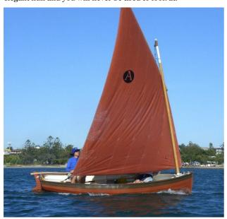
Aber was initially designed for strip planking over laminated or stem bent frames. Now, she may also be clinker planked with 6 mm thick plywood, giving a lighter hull. Aber keeps the look of an authentic traditional construction, with ribs, knees, seat risers. The sheerstrake is usually made of timber and may be varnished. Therefore, nobody will notice that the other planks are made of plywood.
