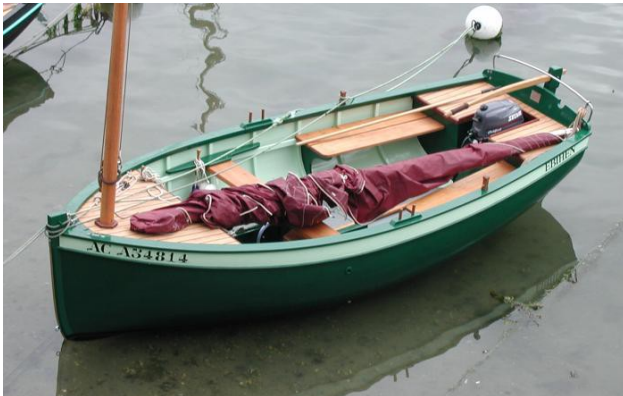
First strip planked Ebihen 15, standing lug rigged
