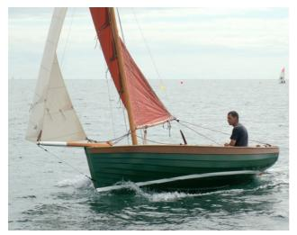
Beg-Meil is a traditional day-boat, gaff sloop rigged, just like many that existed in the old days. It is elegant and seaworthy with its half-deck and varnished wood coamings. A steel pivoting centreboard (40 kg) improves stability and gives excellent windward abilities. Hull shapes are the same as Ilur. Ilur is a reference sail and oars boat, with nearly 1000 plans already sold.
