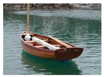
Aber was the first boat created in 1985 as a result of the desire to provide a boat especially designed for the home builder. It is derived from Aven, my first sail & oars design. It is a little smaller, but has more buoyancy in the fore sections for better sea keeping. Aber kept the simple but so efficient lug rig in the Breton style. The rudder is fixed but can slide vertically.
