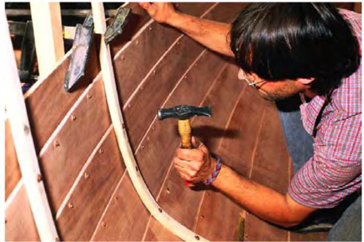
Construction of an Ilur with lapstrake and bent frames: peening rivets. © Francis Holveck in Douarnenez
