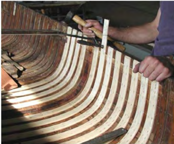
Restoration of a canoe: we use nail bent over on very flexible ribs (of slender thickness)
