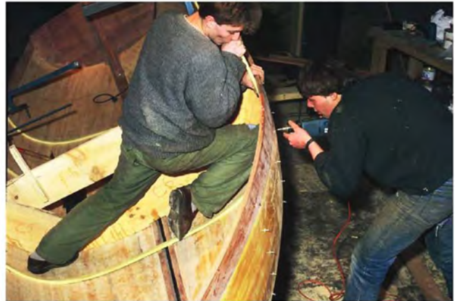
Laying a chord on an Aber, screwed to the plating © Francis Holveck in Douarnenez
