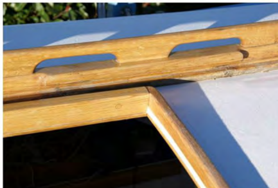
Angle ahead of the hatch showing the continuity of the coaming, which is not interrupted by the slide as is sometimes the case.
