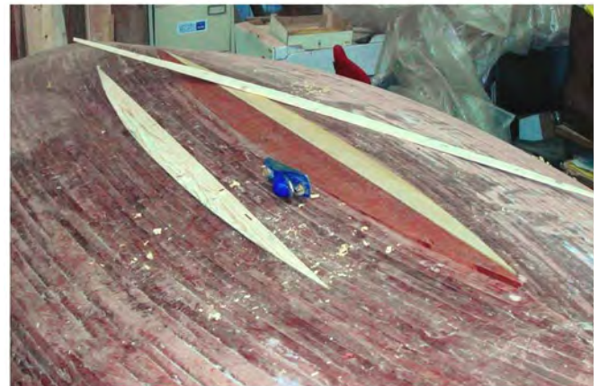
On this Ilur, adjusting the closing plank of solid wood © Jean-Francois Dockes
