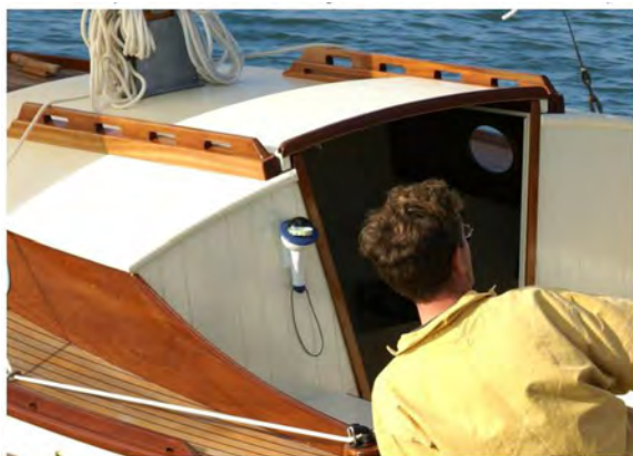
Overview of the descending panels on a Méaban The slides are external to the sliding panel Note the handrails, useful on all boats
