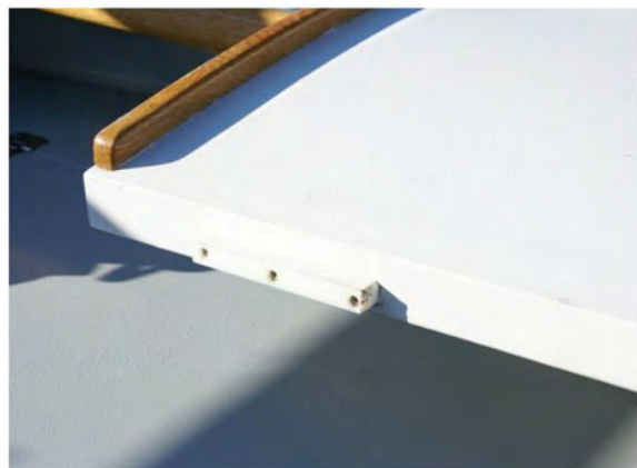
Sliding cleat made of synthetic material, here POM-C (polyacetal copolymer) which slides well and wears little.
