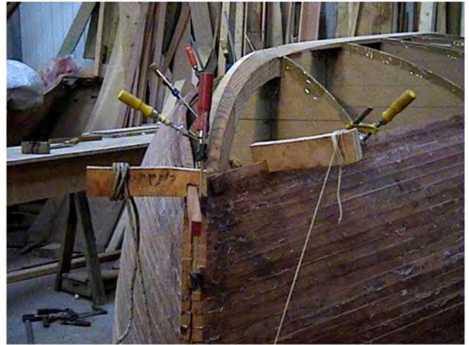
Wooden levers to facilitate twisting the strips © Jean-Francois Dockes
