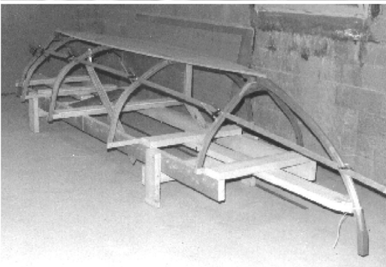
Youkou-Lili: frame construction with sole. The pointed rear is treated exactly like the bow. A batten is presented to check the squareness of frames and bow
